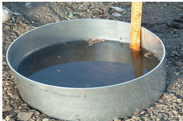
Single ring infiltrometer
