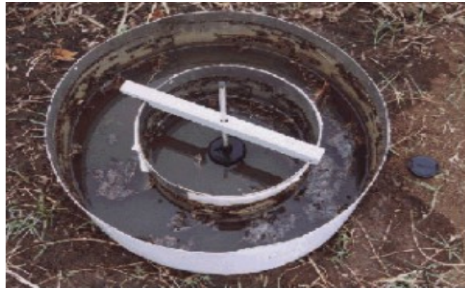
Double ring infiltrometer
